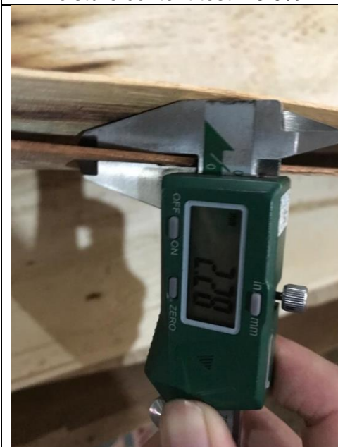
Veneer thickness check: 2.28mm
