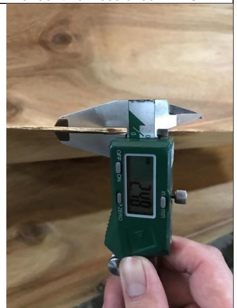
Veneer thickness check: 2.48mm
