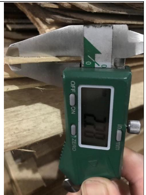
Veneer thickness check: 2.28mm
