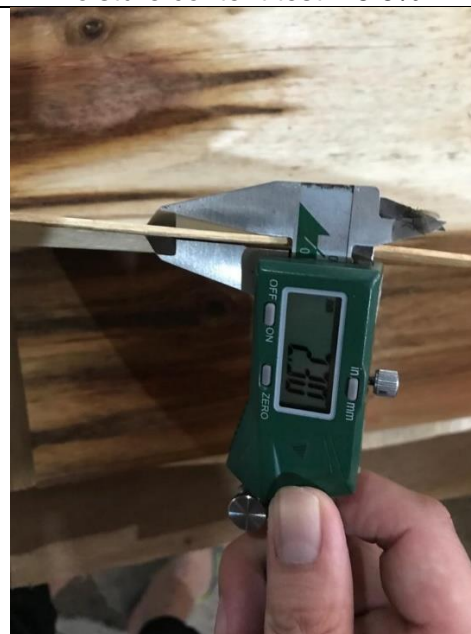
Veneer thickness check: 2.30mm
